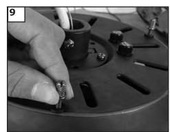
Loosen 3 thumb screws with key hole slots.
